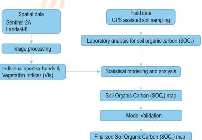
Interpretation: The NDVI and BSI (for L8 data) and BSI and RSR (for S2A data) were found most suitable VI in the prediction of SOC. The R<sup>2</sup> values of linear regression models were 0.68 (BSI) and 0.78 (RSR), indicating that nearly 68% and 78% of the SOC could be predicted through L8 and S2A datasets, respectively.
