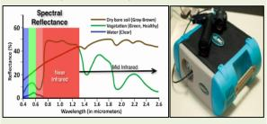
5. Plant Canopy Analyzer (LAI-2200): Used for nondestructive measurements of Leaf Area Index (LAI).
