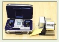
13. Leaf Porometer (SC-1): Measures the stomatal conductance of a plant leaves.
